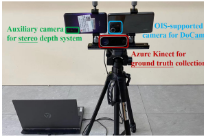
Figure 8: Experiment setup: DoCam, stereo camera system, and Azure Kinect
